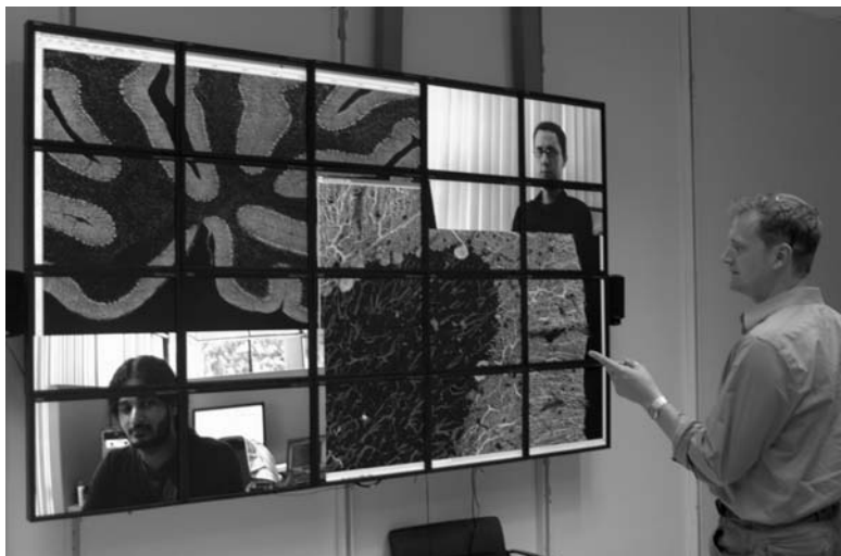
Figure 14.9 SAGE driven high-resolution displays allow users to arrange large datasets next to each other for visual comparison. Collaboration tools in the environment also support HD video conferencing.
