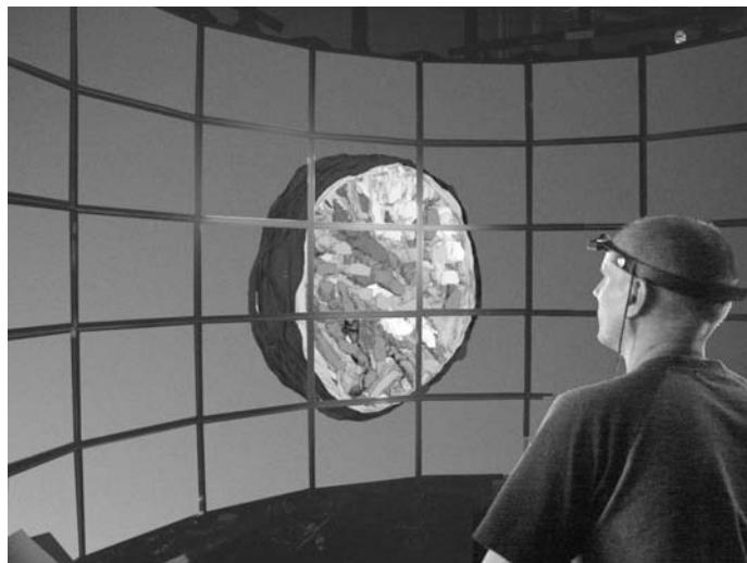
Figure 14.11 (a) How the barrier linescreen technology is used for generating pixel sets which are only visible to one eye at a time. Two such sets enable stereo vision. (b) A user interacting with the stereo display without using glasses.
